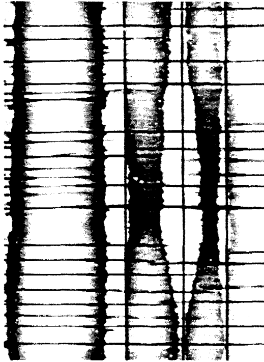
Fig. 1. Typical delamination cracks originating from transverse cracking (Lim, 1988) (white areas represent the delamination zone and solid lines the transverse cracks).
